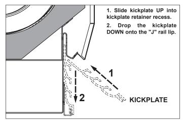
Fig. 8 Kickplate installation
