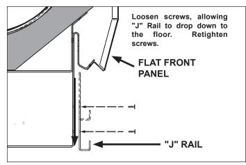
Fig. 7 "J" rail installation
