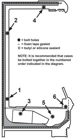
Fig. 2 Bolt holes, foam tape gasket and sealant
