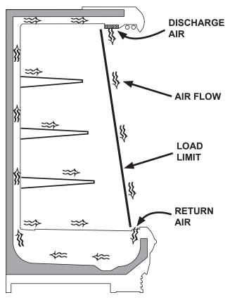
The discharge air probe monitors the temperature of the discharge air and may be used as the defrost termination sensor. The probe can generally be found behind the rear baffle, in the upper baffle, or in front of the honeycomb. NOTE: if the discharge air probe is used for defrost termination, none of the termination sensors listed earlier will be installed in the case.
