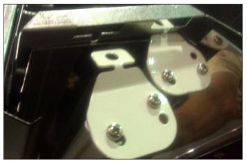
Fig. 22 Slide the other end to the opening in the sheet metal and disengage
