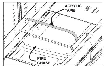
Fig. 4 Sealing the pipe chase
