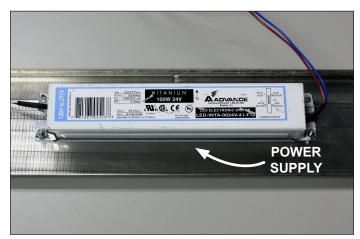
Fig. 23 Clear view of the power supply on the back side of the light reflector
