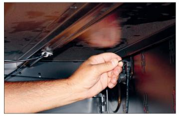
Fig. 19 Unplug the LED luminaire
